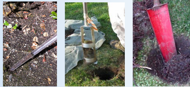
A soil sampling probe, auger or shovel can be used to collect soil samples. Remove surface vegetation before collecting the sample.
