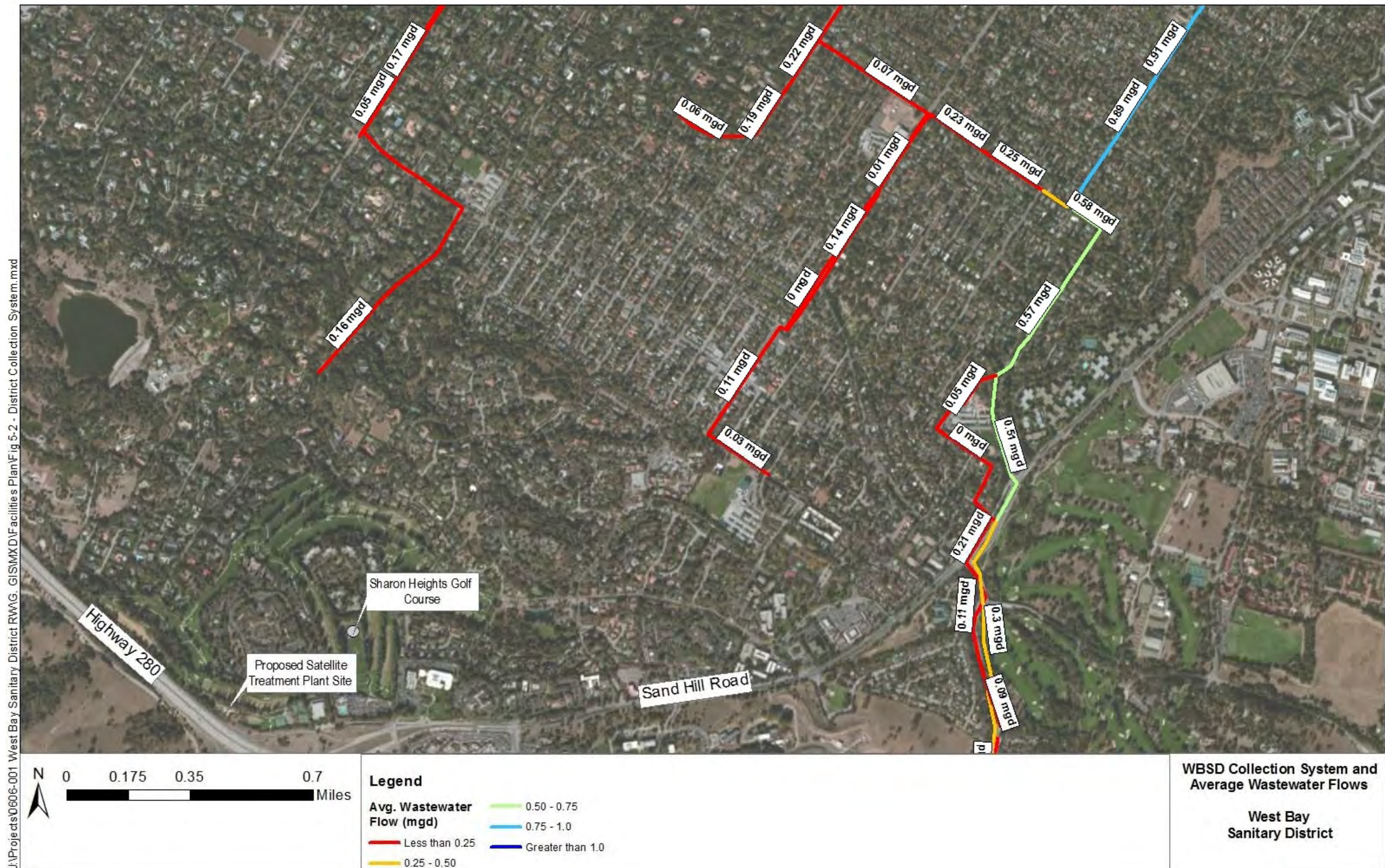
Figure 5-4: District Collection System in Sharon Heights G&CC Area and Average Flow
