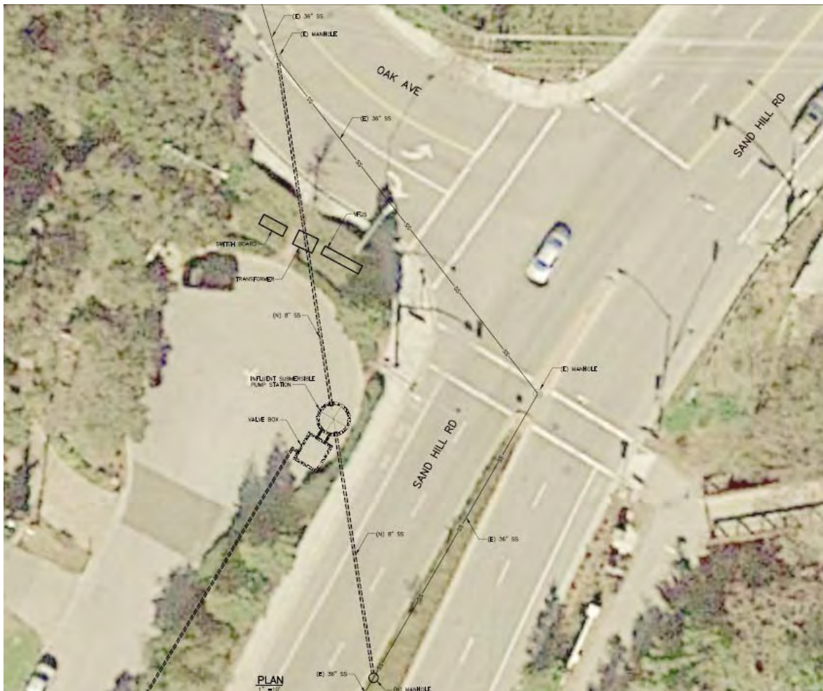
Figure 2.2-4: Wastewater Pump Station Facilities
