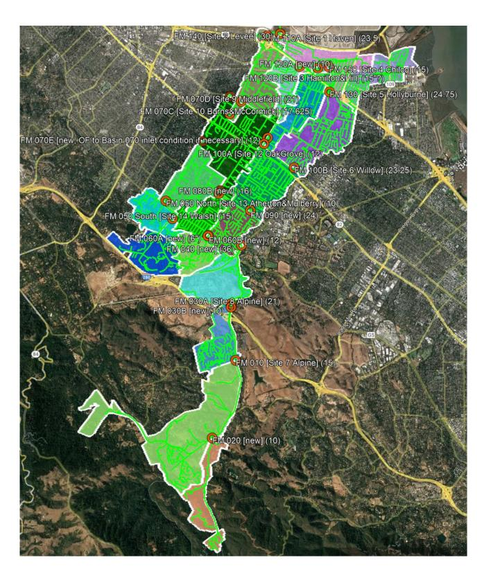
New Flow Meter 020 (expected 10" line) that will capture approximately 70% of the original 020 basin. The northwest portion of the original 020 basin flows into Basin 010. The single flow meter will be stand-alone and capture the entirety of the proposed basin area. Basin 020 Isolation = FM 020
