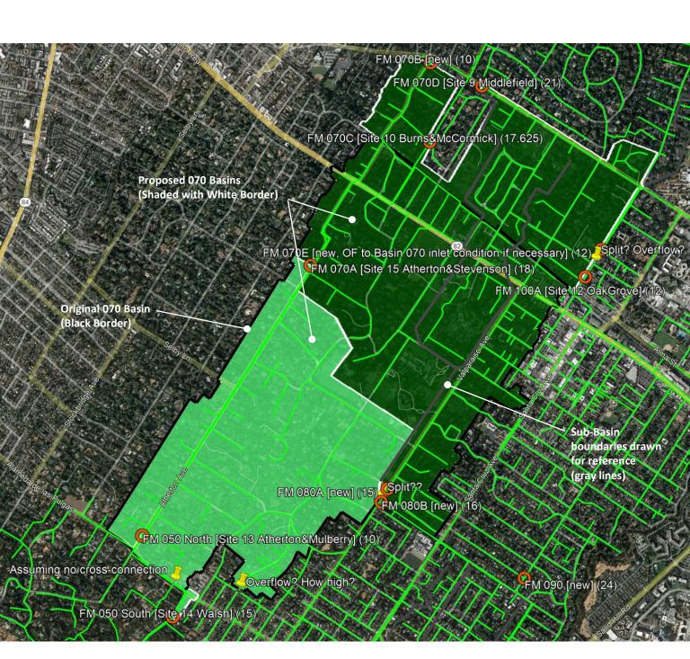
Propose <u>new</u> flow meters 080A (expecting 15" line) and 080B (expecting 16" line) that will capture ~95% of the original 080 basin. There currently are no WBSD meters that measure near this basin. There appears to be a split at Valparaiso, just north of Politzer Drive that necessitates the use of two flow meters to meter this basin.
