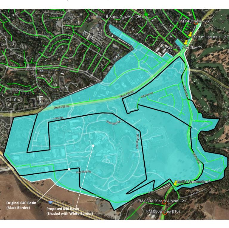
Uses existing Flow Meter 050 South (Site 14 Walsh on 15" line) and uses existing Flow Meter 050 North (Site 13 Atherton/Mulberry on 10" line) that captures ~100% of the original 050 basin, but naturally splits the basin into north and south sub-basins based on existing flow meter locations. A potential cross-connection needs to be confirmed to be inactive.
