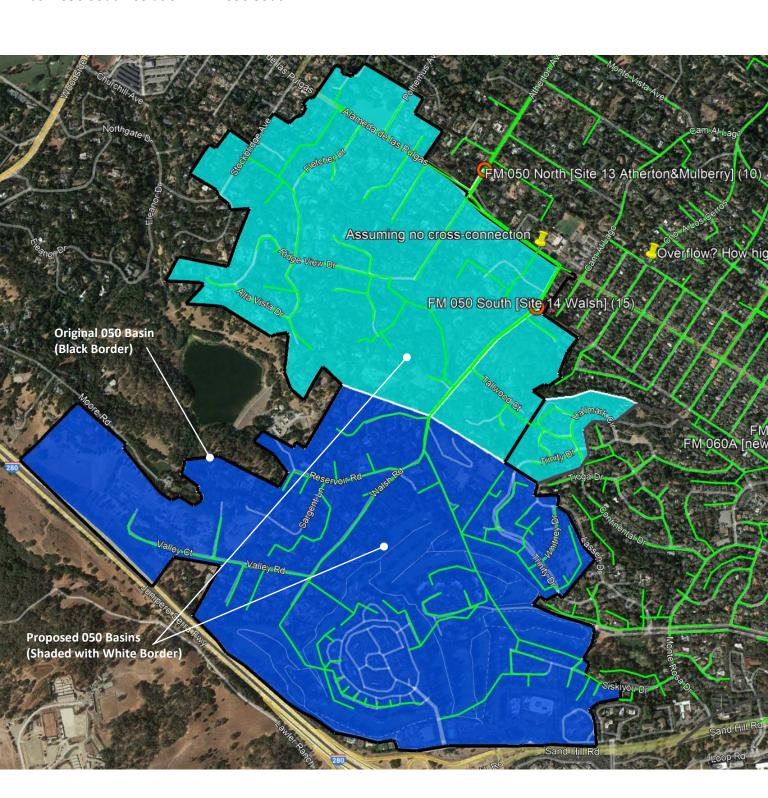
Propose new flow meters 060A (expecting 6" line) and 060B (expecting 12" line) that will capture ~85% of the original 060 basin. There currently are no WBSD meters that measure near this basin. There appears to be a possible split at Altschul/Avy that necessitates the use of two flow meters to meter this basin. It's possible a plug could be utilized as well to achieve basin isolation.
