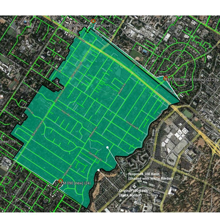
Uses <u>existing</u> Flow Meter 110 (Site 1 Haven on 23.5" line) to isolate Basin 110, capturing ~85% of the original 110 Basin.
